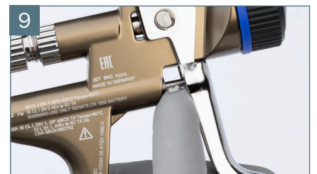
Grease visible part of air piston rod
