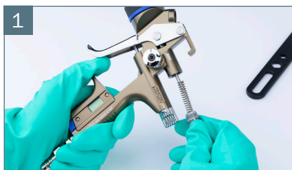
1 First remove paint needle.
